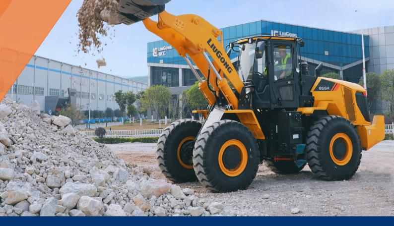
EngineCummins 6LT9.3Gross Power162 kW (217 hp / 220 ps) @ 2,000 rpmNet Power149 kW (200 hp / 202 ps) @ 2,000 rpmOperating Weight18,145 kgStandard Bucket Size3.0 m³Standard Breakout Force148 kNStandard Dump Clearance4,272.5 mm
